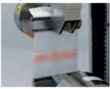
In seam strength tests performed in accordance with EN ISO 13935-2, mechanical pulling force is applied to the material to determine the level of force required to rip the seam.
