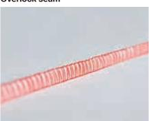
The internal overlock seam is up to 50% more resistant to stress and up to 50% more elastic than quilted seams.
