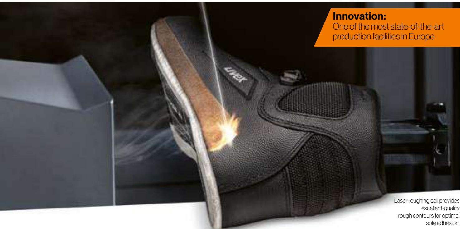
Laser roughing cell provides excellent-quality rough contours for optimal sole adhesion.
